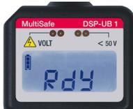
If no „rdY“ appears, the earth connection must be checked and, if necessary, cleaned, and the test probe and electrode checked. The self-test must be repeated.
